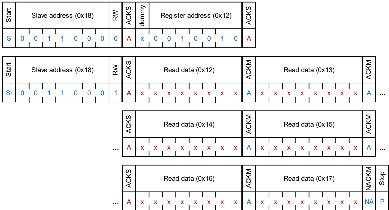
Figure 5: I 2 C multiple read
